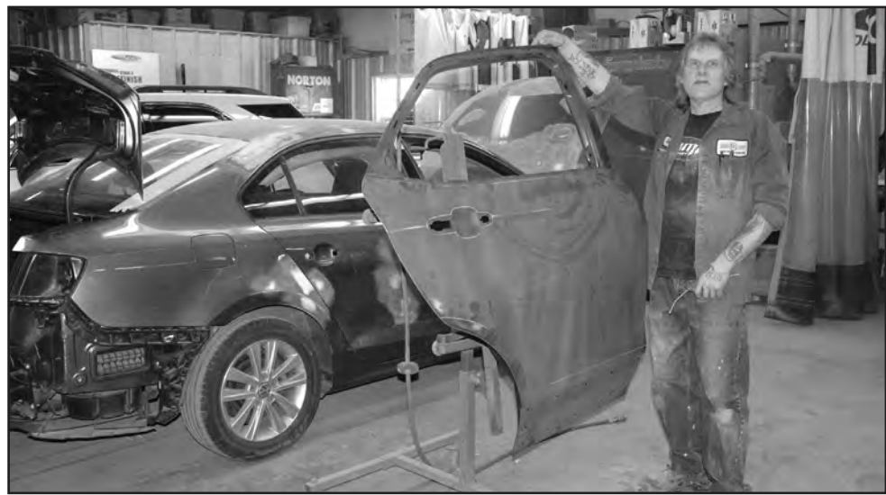
Darren Bracken is working on repairing and getting ready to paint this car door panel.
