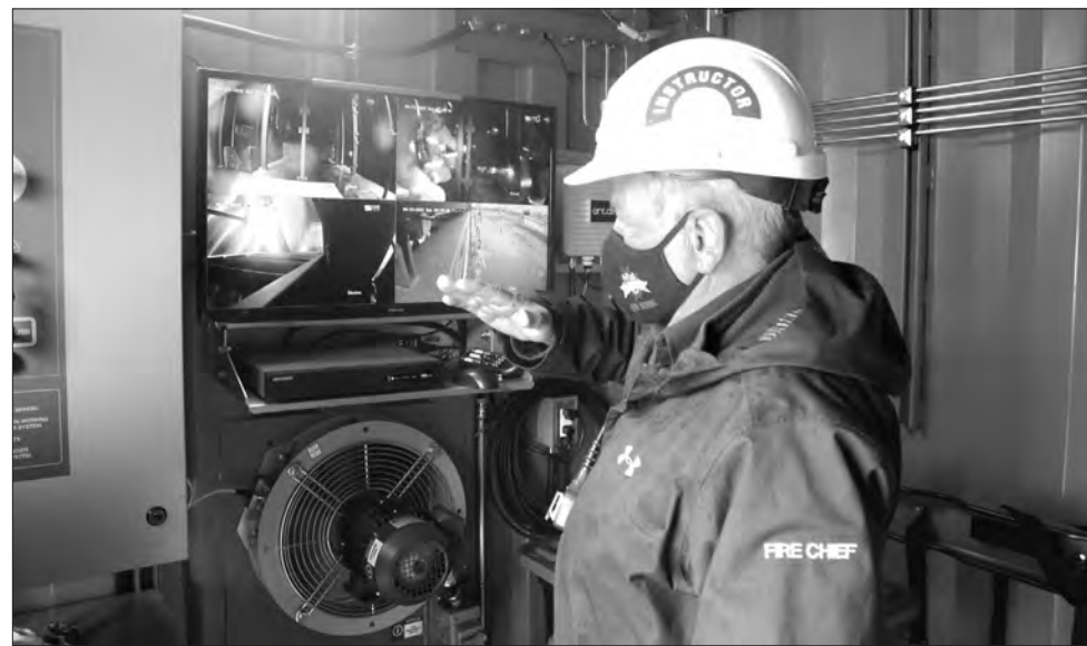
Instructor Graham Warburton explains how the control centre works. He can see on the monitor what is happening inside the mobile unit. He will use a control panel to create different situations within the unit. Another instructor, Jamie Meyer stays with the firefighters and follows them as they go through the unit. Morin Photo
