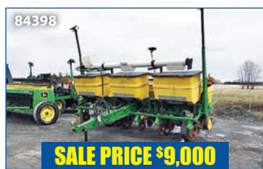
84398 SALE PRICE $9,000 JD 7200 corn planter, 6 row, dry fertilizer with extensions, seed box extensions, cross auger, finger meters. List Price $14,900
